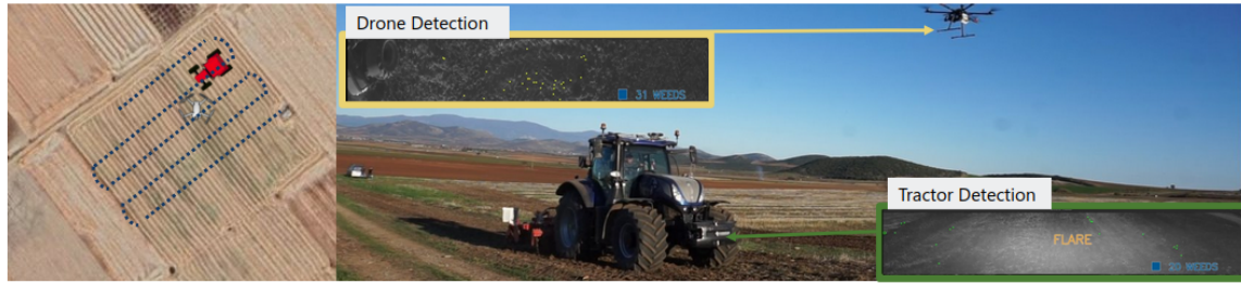
Figure 35: On the left, the tractor's trajectory; on the right, an on-site photograph showing the detection of each component. The tractor's camera is exposed to the sun, and the drone is on its mission to maximize weed detection performance.
